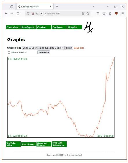
If data logging is active, viewing the Graphs page stops the logging and sets the log interval to No Log.
